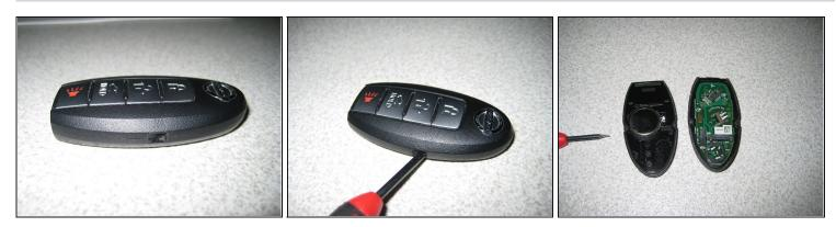
• Insert the small flathead screwdriver into the small notch on the left side of the key fob and carefully pry apart.
