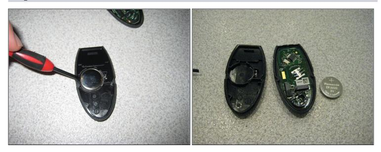
• Pry out the old CR2032 3V battery with the flathead screwdriver.
