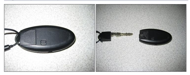
Slide the switch on the back of the key fob and release the physical car key that is stored inside.
