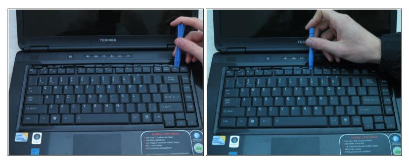
Pry the top of the keyboard loose from its casing using a plastic opening tool.
