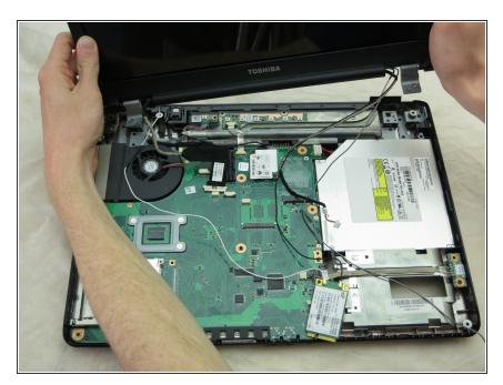
Remove the display assembly and put it aside.
