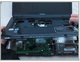
Separate the laptop upper casing from the lower casing by using an opening tool around the sides
