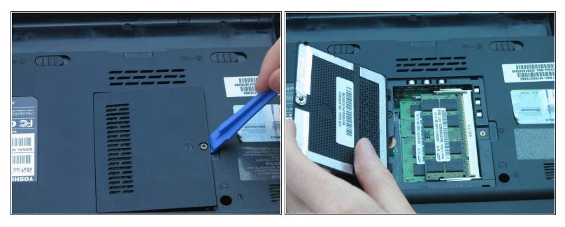
Remove the RAM cover by inserting the plastic opening tool into the indent and lifting.
