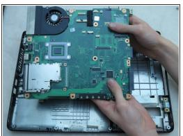
Gently lift the top right side of the motherboard. Pull it upwards to the right and away from you.
