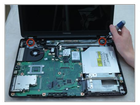
Remove the four 6-mm screws from the two hinge pads using a Phillips #1 screwdriver.
