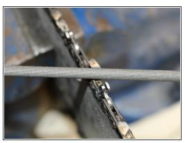
Inspect the tooth and determine which angle to position the file for sharpening. Make sure that the whole tooth of the blade is flat against the file.
