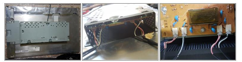
• Lift up the metal bracket and carefully remove all connectors
