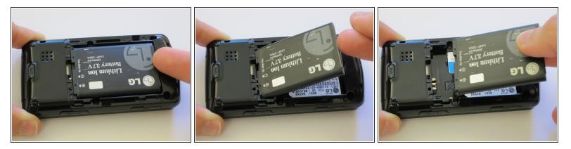
• Take out the battery by levering it out towards the bottom of the phone.
