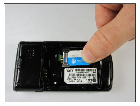
Slide the SIM card towards the bottom of the phone by firmly pressing down on the card. This will remove the SIM card.
