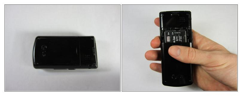
• Use your thumb to press down and slide off the back cover of the phone.
