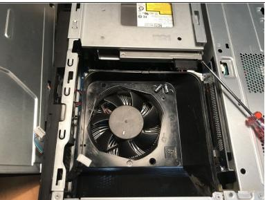
Using a #0 Phillips screwdriver, remove the screws connecting the fan cover to the fan by rotating the screwdriver counter-clockwise. Lift the fan cover out of the desktop and place to the side.
