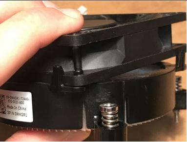
Place the new or cleaned fan onto the heatsink, and press down on the corners to lock the fan onto the heatsink.
