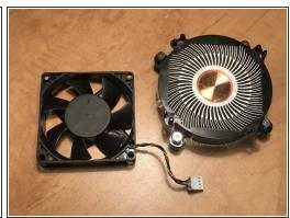
Using your thumb and forefinger, pry off the four clips holding the fan to the heatsink.
