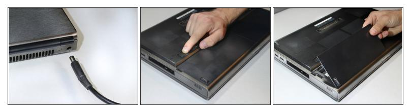
A Ensure that all electrical sources are removed and turned off.
