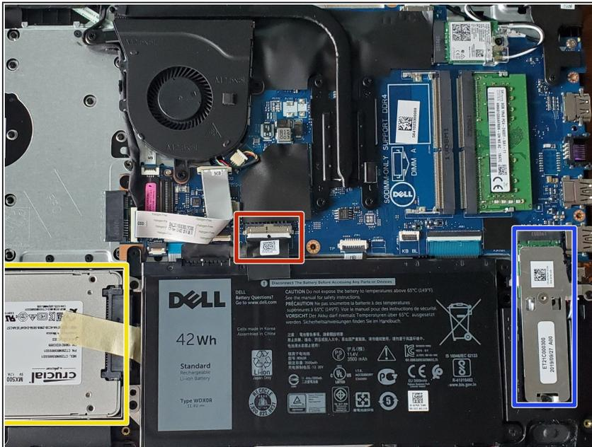
**⚠** It is recommended that you disconnect the battery. Just pull on the tab towards you without lifting up. This is marked in red.
