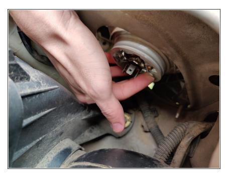
Push down on the metal lever to release it. After you have released the lever you can remove the bulb.
