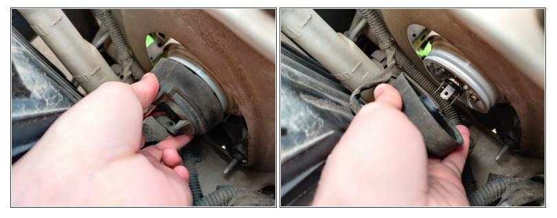
Pinch the rubber cover and disconnect the headlight bulb.
