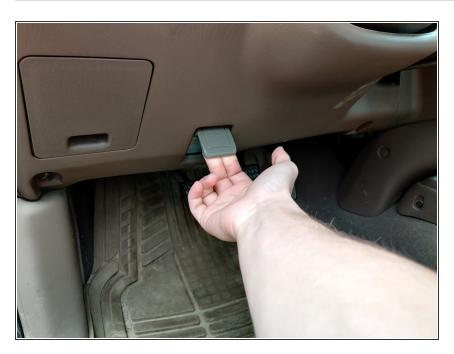
Pull the lever under the steering wheel.
