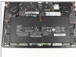
Remove the five 3.6 mm screws from the battery with a Phillips #00 screwdriver.
