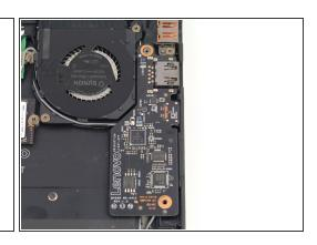
Remove the single 3.6 mm screw from the daughterboard with a Phillips #00 screwdriver.
