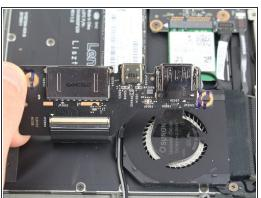
Grabbing the outside edge of the daughterboard, flip the board up to reveal the ZIF connector on the underside.
