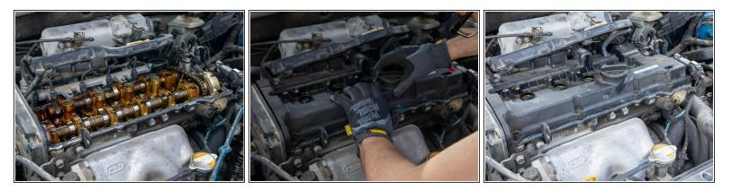
• Place the engine head back on the engine.
