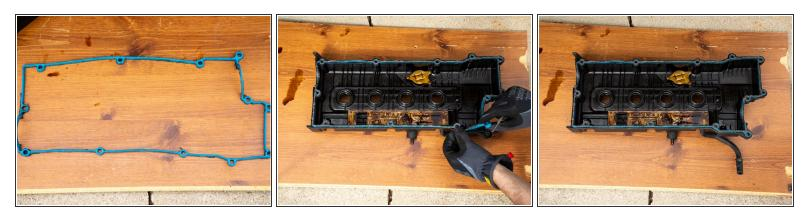
• Insert the engine block seal into the engine head.
