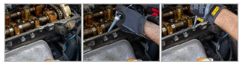
• Clean the residue off of the engine block.
