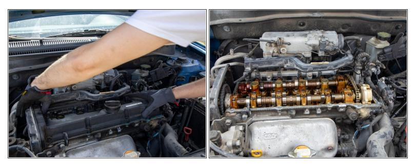
• Remove the engine head.
