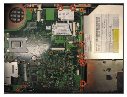
Remove the six 4mm flat-head screws with a Phillips 00 Screwdriver.
