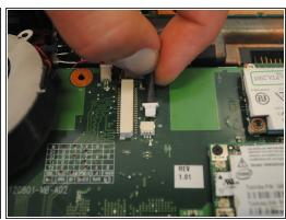
• Locate and remove the smaller white connector (far right) and any tape that is holding it down.
