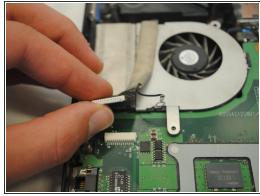
• Locate and remove the white connector that is .75 inches wide.
