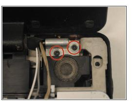
Remove the four 8mm button-head screws that are located in the top right (2) and top left corners
