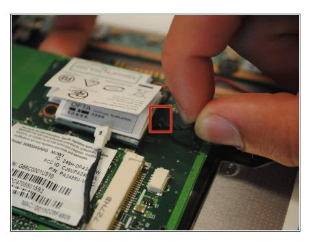
Locate the black wire next to optical drive and gently pull it away from the socket to remove it.
