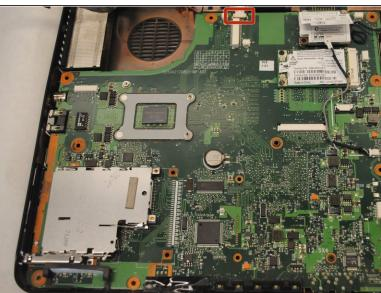
Pinch the plastic cable horizontally and pull it away from the socket in order to remove the cable connecting the motherboard to the speaker cover buttons.
