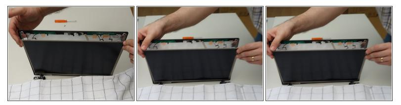
• Cover the keyboard with a cloth, then carefully lower the LCD screen onto the keyboard.
