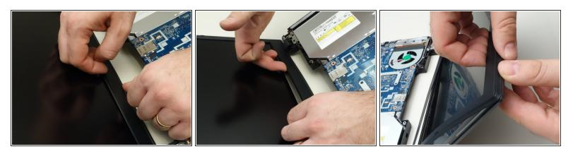
Working your way around the frame, unclip the mounting points of the frame surrounding the LCD screen.
