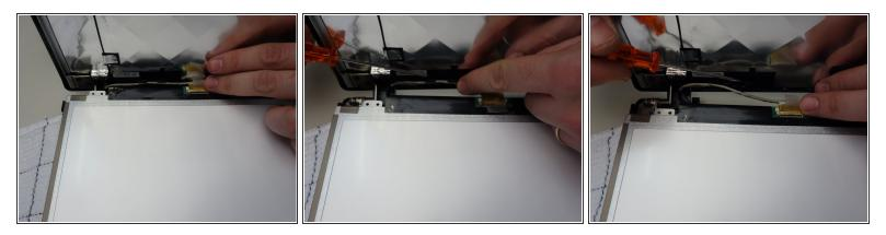
• Using the plastic tab, peel back the tape securing the LCD cable the panel connector.
