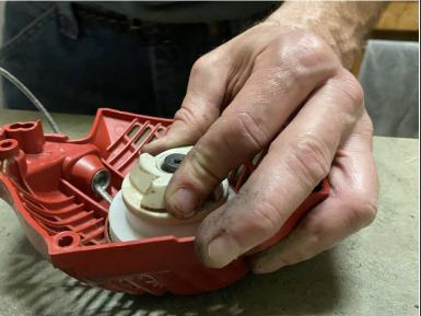
Slowly rewind the housing unit until the rope is back into its original position.
