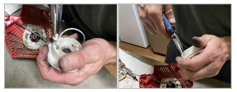
Remove the rope from the chainsaw using a pair of pliers.
