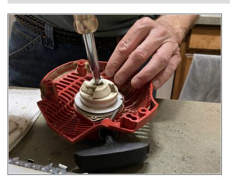
Remove the screw on top of the housing.
