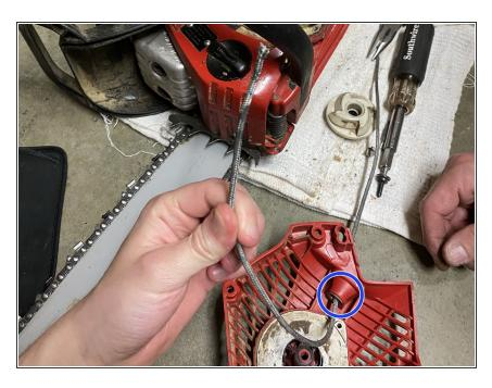
Stick the rope back through the insertion hole.
