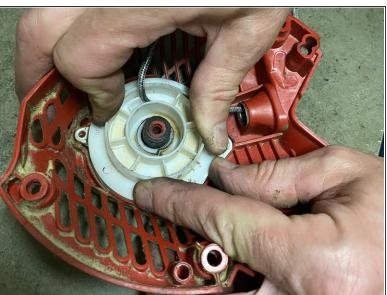
Stick the rope through the groove into the housing.
