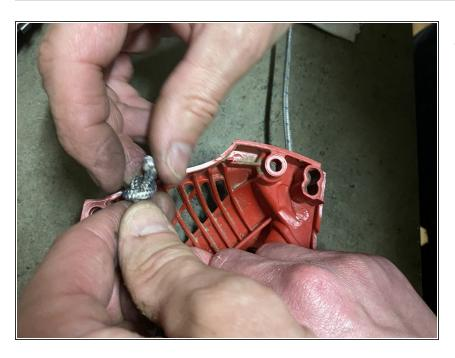
Re-tie the rope into a knot.
