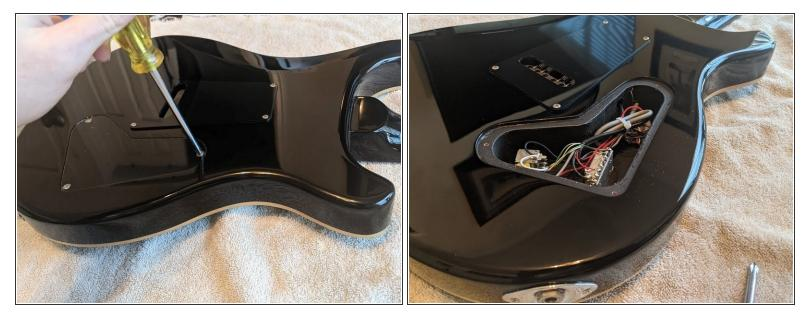
Using a Phillips head screwdriver, unscrew the back plate, revealing the pickup wiring.
