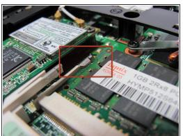
Pull apart the two tabs holding the RAM in place.
