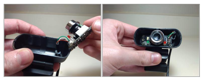
• Place the motherboard and camera back into the casing.
