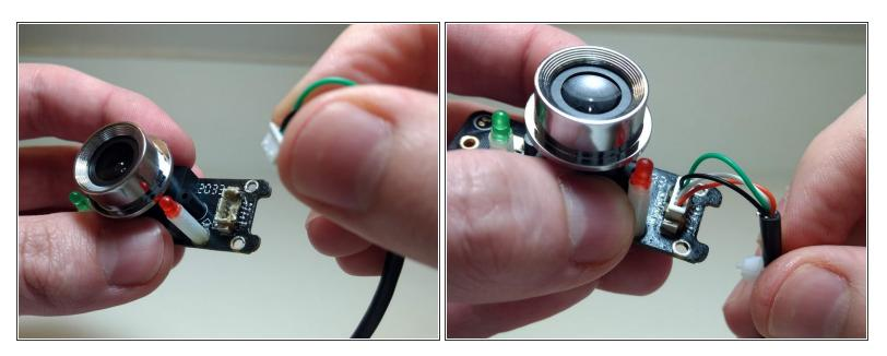
• Reattach the cable to the connector.
