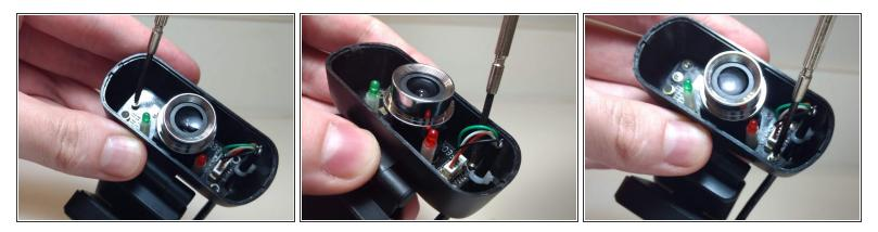
• Screw the camera and motherboard back into place.
