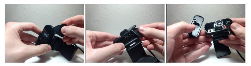
Pry open the face plate of the webcam using the iFixit opening pick or another safe tool, and set it aside.
