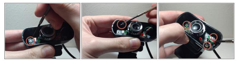
Remove the three main screws using a Phillips screwdriver while carefully holding the camera motherboard in place.
