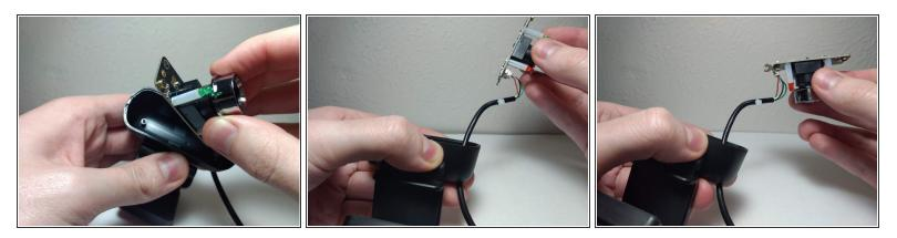
• Remove the camera and motherboard from the casing carefully.
