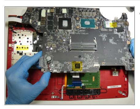
Gently lift away the motherboard, directly upward.
