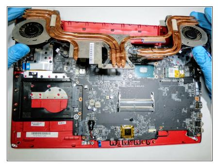
Remove the heatsink from the device.
