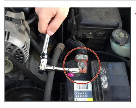
Disconnect the positive power connection (red) with a 3/8" ratchet and a 1/2" socket.
