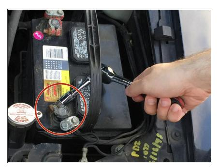
Disconnect the negative power connection (black) with a 3/8" ratchet and a 1/2" socket.
