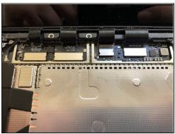
• Remove the clip-on shields for the display assembly.
