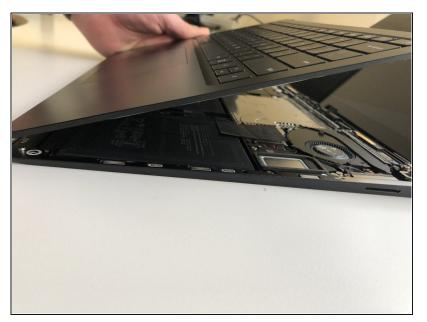
With the screen open, lift the keyboard out. It doesn't take much force as the part is only held in with magnets once the screws are removed.
