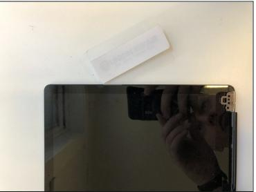
• Use a metal card to get in between the glass and the housing. Swap to a <u>plastic card</u> to cut through the rest of the adhesive.
