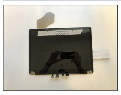
Watch out for the Sensors up the top. If you damage these the device will fail to turn on. It basically bricks completely without the sensors.
