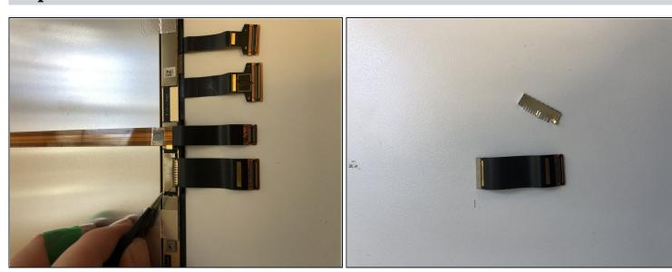
• Remove the snap-on shield and cable. We will need this later.
