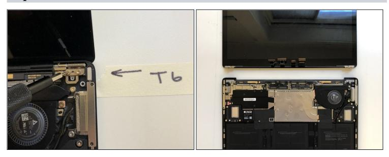
• Using a T6 screwdriver, remove the 6 screws holding in the display.
