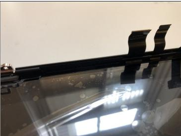
Slide the cable back under the plastic bar and set it back in place. Lightly pull the cables to make sure there's no slack internally.
