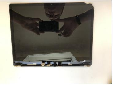
• Heat up the bottom of the display and horizontally pull the screen out. Try to leave the bottom adhesive intact as we are going to be using this later.
