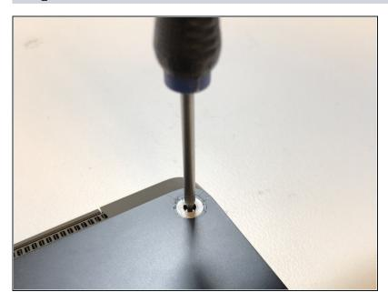
• Using a T5 screwdriver remove the 4 screws on each corner.
