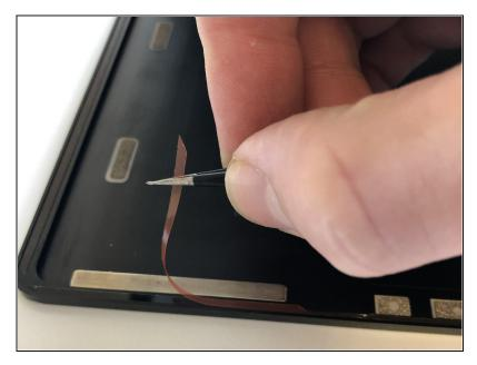
Remove the plastic layer on top of your adhesive and set the screen into the housing. You need to push the screen in quite a bit at the bottom to make it sit correctly.
