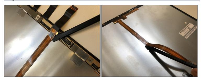
• CAREFULLY loosen the sensor cable on the back of the display.
