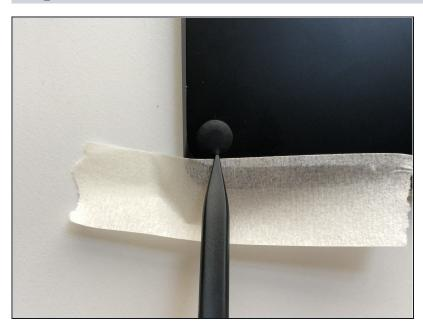
From the bottom, carefully pry up the rubber feet on all 4 corners.
