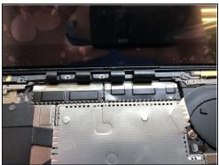
Place the assembly in then screw it in. Connect the cables and replace the shields.
