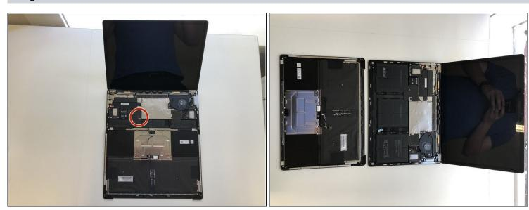
• Invert the keyboard on itself and remove the unshielded keyboard assembly connector.
