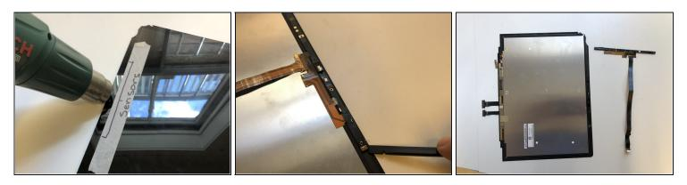
• Heat the area around the sensors from the front. The adhesive here isn't very strong so you don't need loads of heat.
