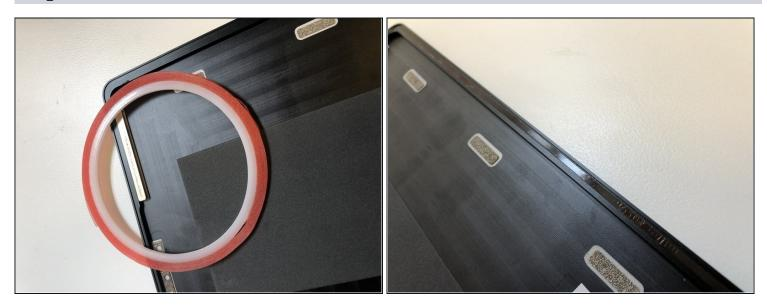
• Install the new adhesive. Remove any large clumps on the bottom. We left the old stuff down there as it's a bit awkward to get to cleaning and reapplying-wise.
