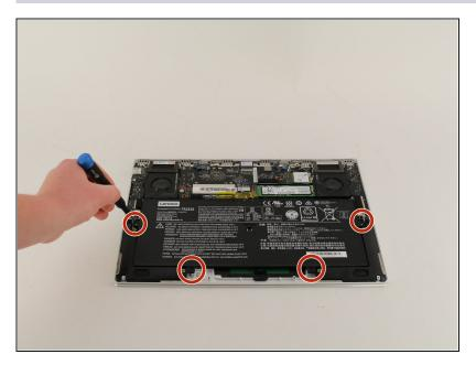
Remove the four 3 mm Phillips #0 screws holding the battery in place.
