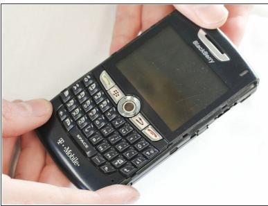
Use a nylon spudger to carefully remove the two side bars of plastic.
