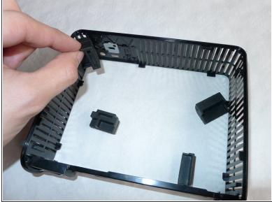
Remove the 4 rubber piece from the plastic frame at each corner.
