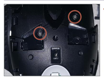
Phillips screws that were revealed after taking off the left and right click buttons
