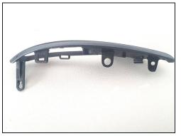
The side cover has several hooks to the mouse housing, look at the images below, and using plastic elements such as Spudger or iFixit Opening Tool, to help you. At the same time you can remove the right click button, which you will see in the next part.
