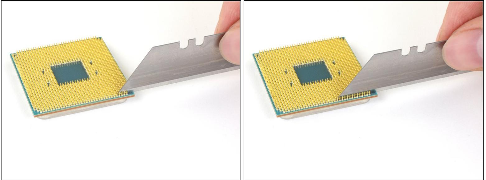
**i** A conventional trapezoidal utility razor blade (like one you would find in a box cutter) fits perfectly between the rows of pins. The thickness of the blade matches the necessary gap between the rows.
