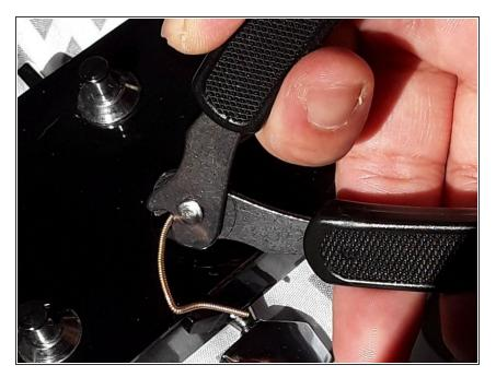
Cut any excess strings on the tuning post using the All-In-1 Restringing Tool's clippers.
