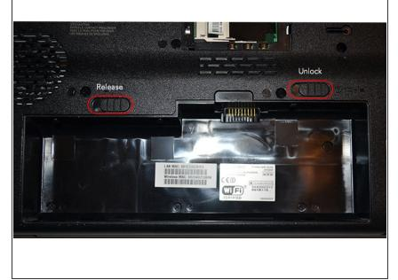
Now that your Toshiba L355 laptop battery is unlocked, find the battery release button down.
