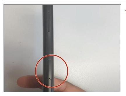
Insert the SIM Card Ejection tool into the small hole and remove the SIM Card tray.
