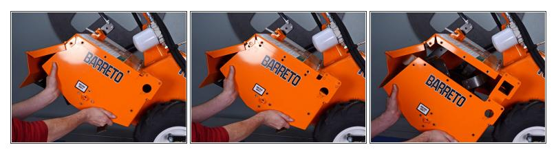
Slide the side plate down and away from the device to remove it.
