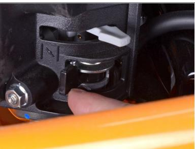
Flip the fuel valve lever to the OFF position.
