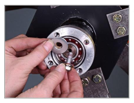
Remove the three washers, held in place by the bolt, from the outboard bearing assembly.
