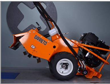
Tilt the tiller up so the motor side is resting on the work surface with the tines raised.
