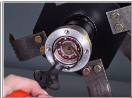
• Use a pair of snap ring pliers to remove the snap ring from the outboard bearing assembly.
