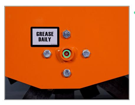
Use an 8 mm socket to remove the outboard bearing grease fitting.
