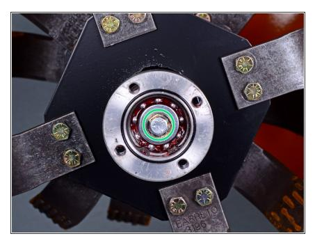
Use a 9/16 inch socket to remove the bolt securing the outboard bearing assembly to the tine shaft.
