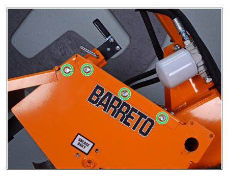
Use a 1/2 inch socket and wrench to remove the four bolts and accompanying nuts securing the side plate to the tine cover.
