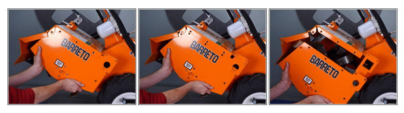
Slide the side plate down and away from the device to remove it.
