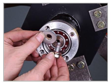
Remove the three washers, held in place by the bolt, from the outboard bearing assembly.
