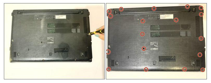
• Remove the seventeen 5 mm screws from the back cover using a Phillips #00 screwdriver.
