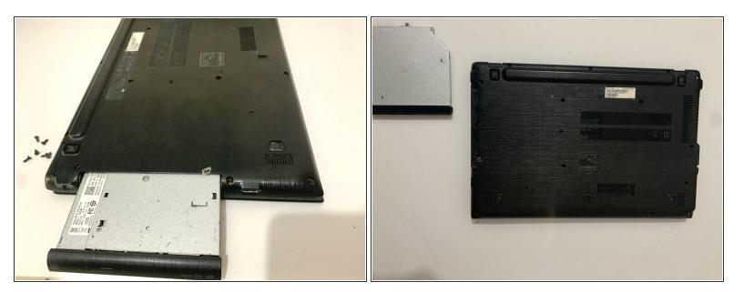
• Remove the CD drive located on the side of the laptop.
