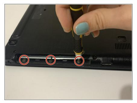
Remove the three 2 mm screws from the disc drive bay using a Phillips #00 screwdriver.
