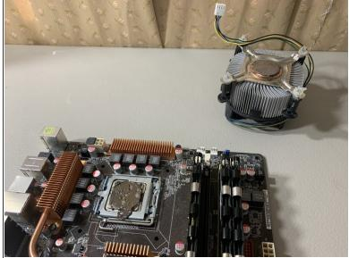
Now remove the CPU cooler off your motherboard, and place the cooler aside.
