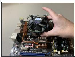
Reinstall the CPU cooler and replace the four pins turning them clockwise to secure it to the motherboard.
