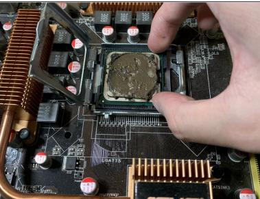
After fixing the pins, gently place your CPU with your thumb and middle finger into the socket.
