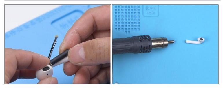
(i) AirPods 1 and 2 have cylindrical batteries that plug directly into the body. We need to use Hot Air Gun with helical wind to heat the metal cap to remove the battery.
