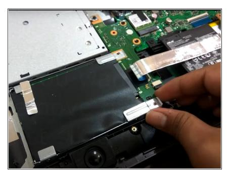
Gently take the left-side board containing the ports by simply sliding it in and taking it out while still connected to the wire.
