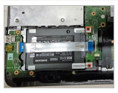
Using the Phillips #0 screwdriver, remove the two 2 mm screws holding the HDD in place.
