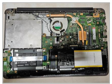
Remove the back cover of the laptop to expose the inner components.
