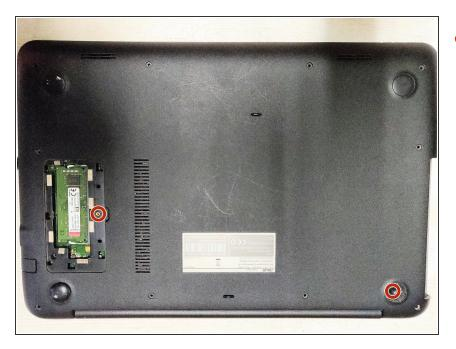
Remove two 2 mm hidden screws using the Phillips #0 screwdriver.
