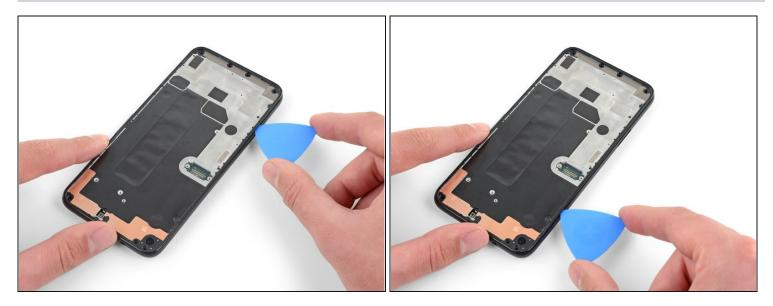
• Slide the opening pick around the left edge of the phone to release the plastic clips securing the back cover to the midframe.
