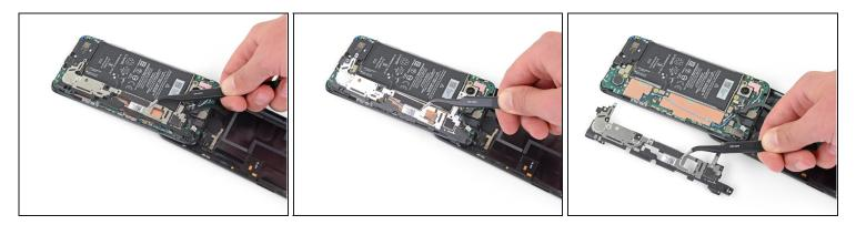
• Use a pair of tweezers to remove the motherboard bracket.
