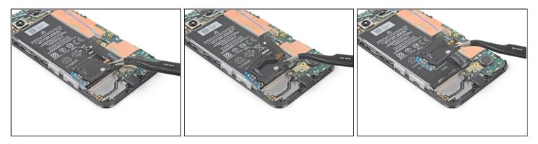
Carefully peel the loudspeaker assembly up off of the tape underneath it.
