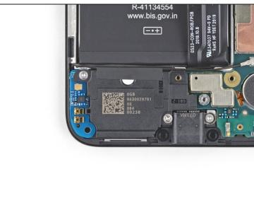
• Use a T3 Torx driver to remove the two 4.1 mm screws securing the loudspeaker assembly.
