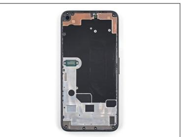
• Use a T3 Torx driver to remove the eight 4.3 mm screws securing the back cover to the midframe.
