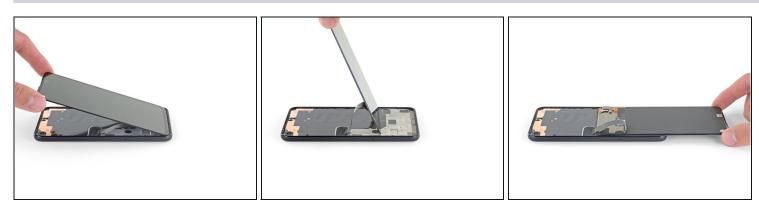
• Lift from the top edge and swing the screen over the bottom edge until you can rest it glass-side down.
