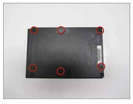
Locate the six feet on the bottom of the PS2.
