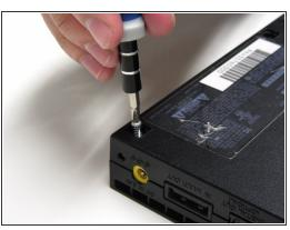
After all of the feet have been removed, Use a Phillips #1 screwdriver to remove the six 4.0mm screws from the base of the PS2.
