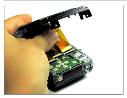
Remove the two LCD board ribbon cables out of their sockets. To reassemble your device, follow these instructions in reverse order.
