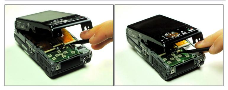
• Using your fingernail or a spudger, flip up the ZIF locking flap on the two LCD ribbon cable sockets that connect the back cover to the rest of the unit.
