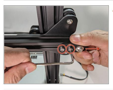
Tighten the belt by pulling on the tensioner bracket as you tighten the two 3mm Allen head screws.
