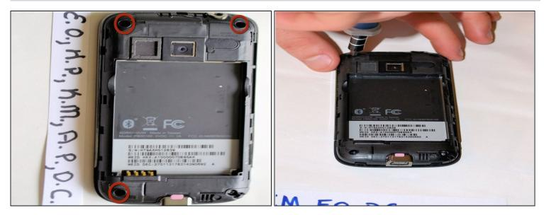
• Use the T4 screwdriver to remove the three .05 mm screws from the back cover.
