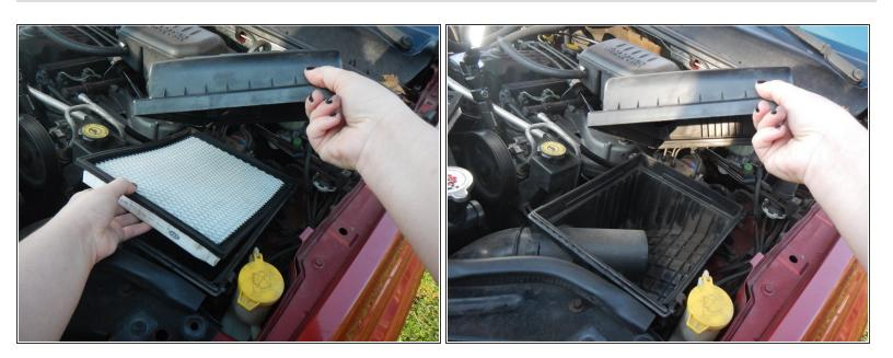
Remove the old air filter and clean any debris out of the bottom half of the housing.
