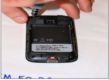
Use the T4 screwdriver to remove the three .05 mm screws from the back cover.
