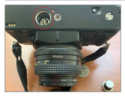
• Replace the battery and battery cover.
