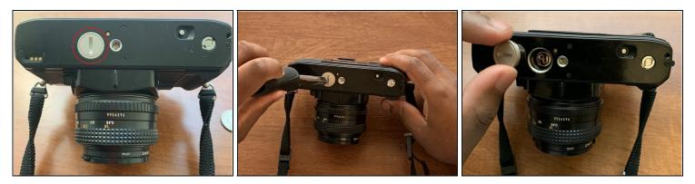
• Using a Flathead screwdriver, remove the battery cap and then remove the battery.
