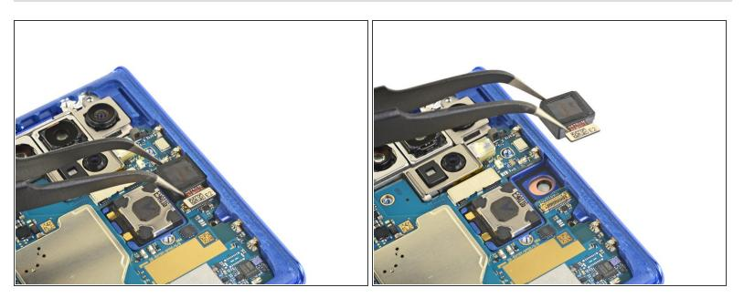
Use a pair of tweezers to remove the front-facing camera.
