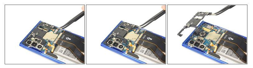
Use a pair of tweezers to pivot the top plastic cover up and off of the phone.
