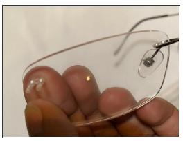
Take the compression sleeves and insert them into the outer lens holes with the pins facing out.
