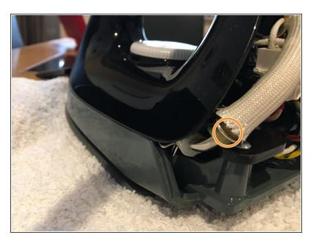
With small pliers locate water tube and squeeze locking ring around small chromed tube (orange), near sole plate and carefully slide away and remove silicon hose from chromed tube.
