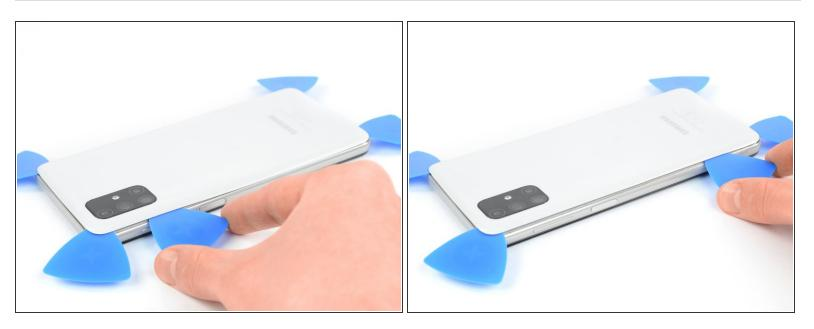
Insert a fifth opening pick on the top left corner and slide it along the edge to cut the remaining adhesive.
