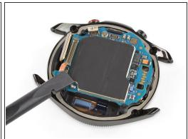
• Use the flat end of a spudger to disconnect the flex cables of the side buttons, the display and the hall sensor.
